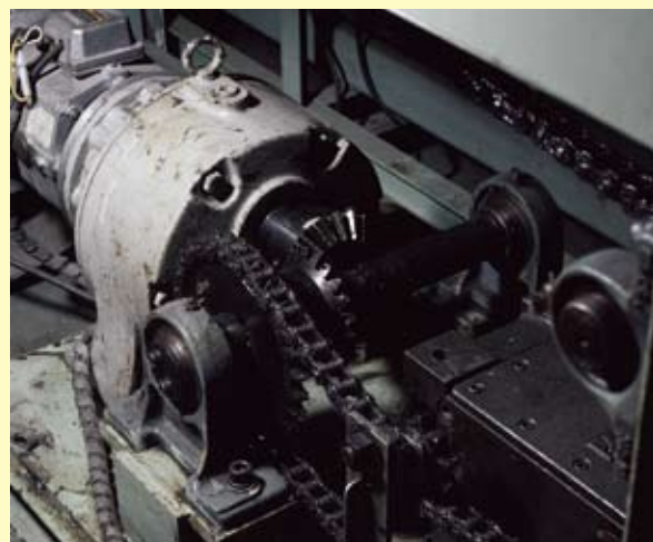
Components of automated line (Bevel Gears)
